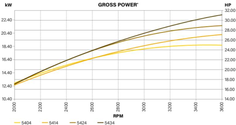
\* All power levels are stated gross kilowatts per SAE J1940 as rated by Briggs & Stratton.
